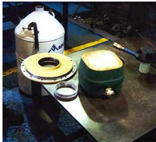
Figure 2: Bearings cooled in liquid nitrogen fit easily and silently into casing.
