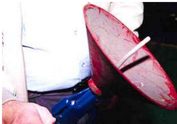
Figure 4: Cup fitted over air gun nozzle.
