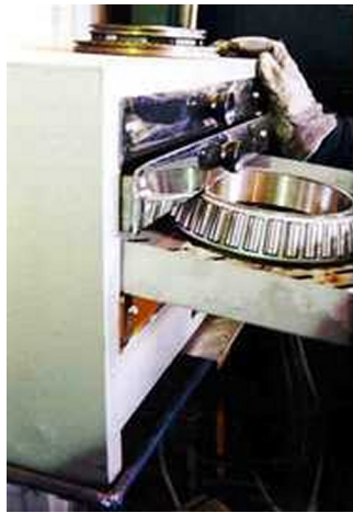
Figure 1: Bearings heated in pie warmer fit over shafts without hammering.
