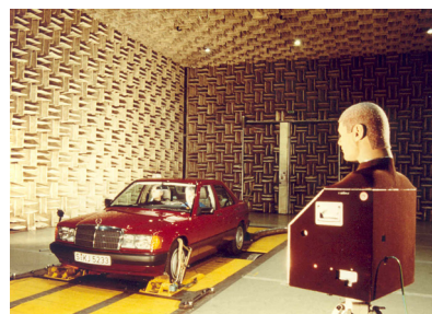
Early representative of artificial head family (named „Gottlieb“) in action at automotive test bench
