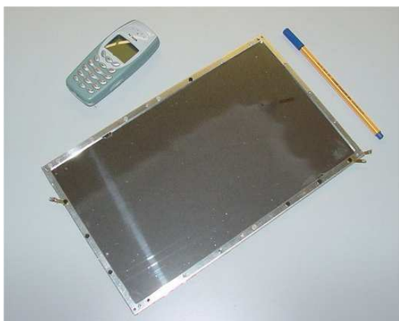
Figure 4: High-power ultrasonic transducer (size: DIN A4)
