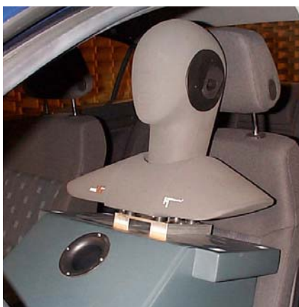
Figure 2: Binaural sound source and additional subwoofer
