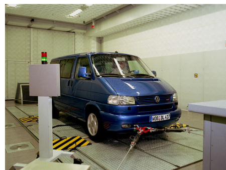
Figure 2: Four-wheel roller test bed with cooling fan.
