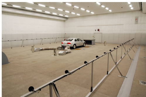
Figure 5: Hemi-freefield pass-by measuring hall (raw volume 3454 m 3 ) equipped with 620 mm deep ASA + CPA anechoic lining in the Acoustics Centre of VW [8] for precision measurements with tonal (sine) sources according to [1].
