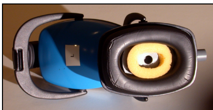
Figure 1: Picture of the right headphone shell containing a plastic piece for the interfacing of the tube. A soft foam ring is inserted to seal the pinna as close as possible to the tube without needing to plug the tube into the ear canal.
