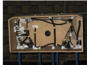
Figure 1: hoses filled model of the engine compartment
