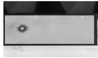
Figure 3: \omega/2 -image of damage in CFRP sample (14,5x4cm).
