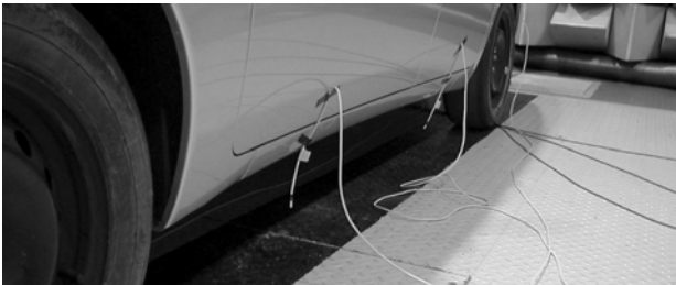
Figure 3: Receiver positions at the left long side of an underneath car cavity.
