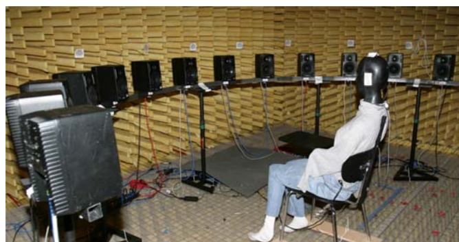
Figure 1: Measurement manikin and speaker setup in the anechoic chamber.
