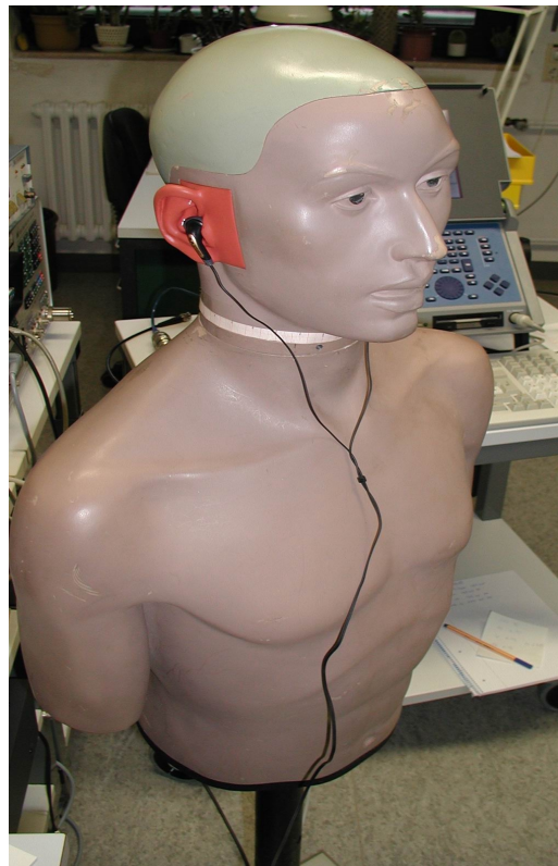
Figure 1: Use of a head and torso simulator for the measurement of eardrum levels.
