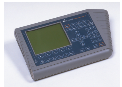
Figure 4: The swept-sine method may be implemented in a sound level meter like Nor121 .
