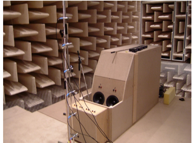
Figure 3: Test rig in the anechoic room of the Institute of Technical Acoustics in Berlin In front the 6 sensors to estimated the far field radiation, two secondary loudspeaker on bogie-shroud with the error sensor in front
