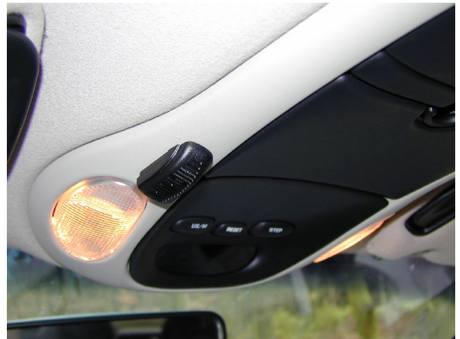
Figure 3: Typical installation of a handsfree microphone
