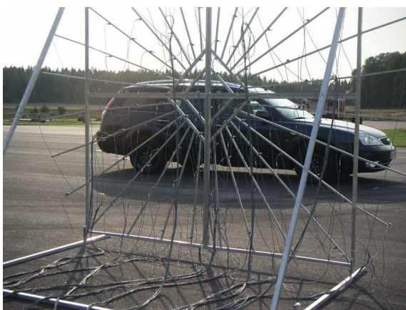
Figure 1: Acoustic camera consisting of about 100 microphones, held in positions by an aluminium stand. A passenger car in the background.
