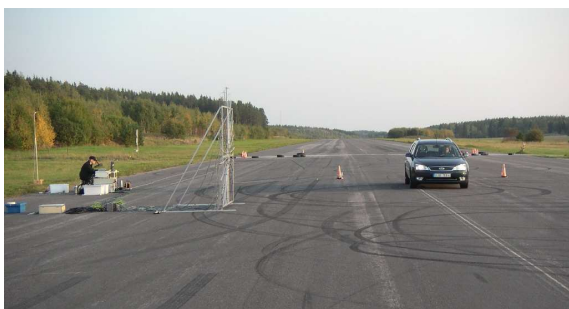
Figure 2: Passenger car passing the acoustic camera at a measurement distance of 5 m, while recording a sound image.
