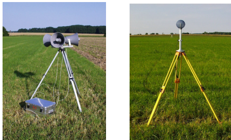
Figure 2: The sound source, a system consist of three compression driver (left side) and the receiver unit (right side), a microphone with a wind screen.
