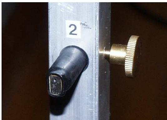
Figure 1: Detail of a tube-mounted silicon microphone.
