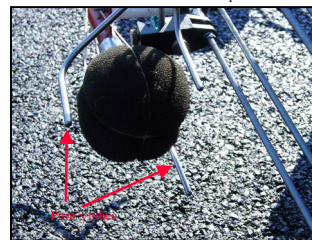
Measurement of airflow speed around microphone windshields
