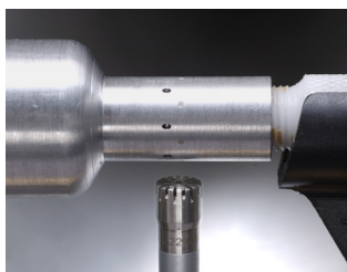
Figure 4: Two cavities system. A 1/4” microphone is put in front of the holes. On the right we can see the support of the microphone encapsulated in the high frequency cavity (Mach wave) and on the left the more important volume of the cavity dedicated to low frequencies (muzzle wave).
