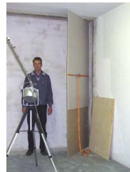
Figure 4: Gypsum board in the corner to change radiation conditions of the test wall
