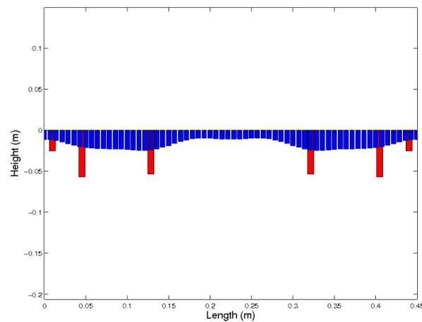
Figure 3: Optimization solution 2 ( $M_n^*, L_n^*$ ). Blue: original bar profile; Red: additional tuning masses.
