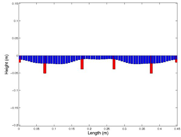
Figure 2: Optimization solution 1 ( $M_n^*, L_n^*$ ). Blue: original bar profile; Red: additional tuning masses.
