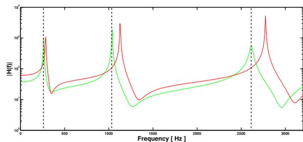
Figure 6: Transfer functions. Red: Unloaded bar; Green: Bar with optimized additional masses.
