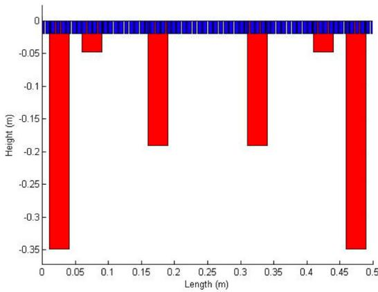
Figure 4: Optimization results ( $M_n^*$ ,  $L_n^*$ ). Blue: original bar profile; Red: additional tuning masses.
