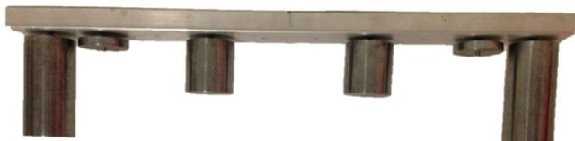
Figure 7: Uniform cross-sectional bar with screwed optimized additional masses  $M_n^*$  at the  $L_n^*$  positions.
