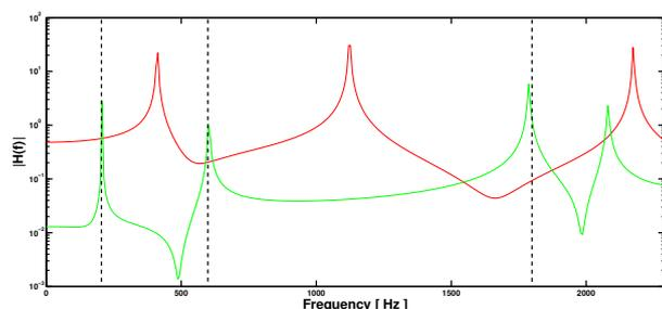
Figure 8: Transfer functions. Red: Unloaded bar; Green: Bar with optimized additional masses.
