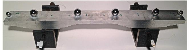
Figure 5: Vibraphone bar prototype with additional masses  $M_n^*$  in the  $L_n^*$  positions.
