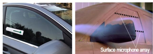
Figure 21 Stick-on/peel-off design of the array - applied to an automobile side glass (left) and showing *in principle* application to clay model in wind tunnel (right)
