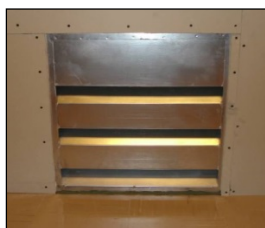
Figure 10 – The non-acoustical grille and commercial acoustical louver tested in the NVOS Lab.
