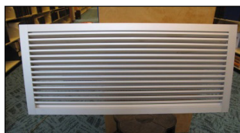
Figure 10 – The non-acoustical grille and commercial acoustical louver tested in the NVOS Lab.
