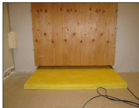
Figure 11 – Slot ventilation opening with 50-mm-thick glass-fibre panel on adjacent, perpendicular surface.
