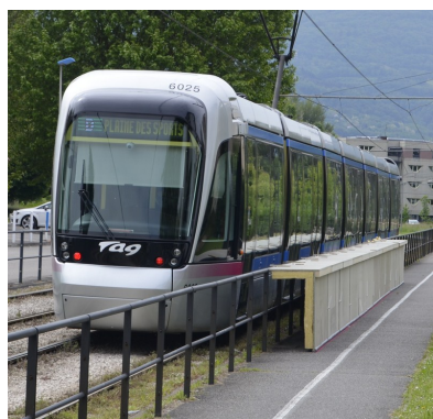
FIGURE 2 – View of the noise barrier prototype with an Alstom Citadis 402 tramway of the Grenoble B line passing-by.
