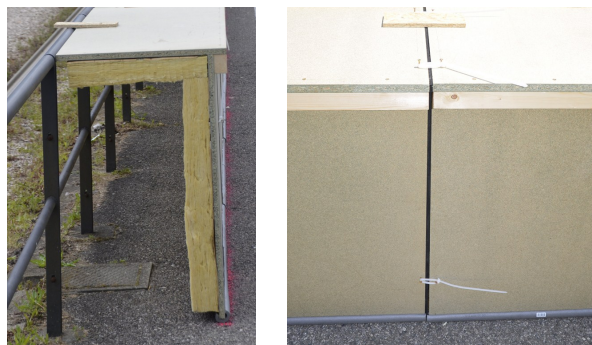
FIGURE 3 – Views of the low-height barrier prototype. Left : cross section. Right : joint system between elements.
