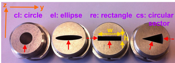
Figure 2: Illustration of experimentally assessed uniform cross section shapes and position of the pressure taps P_1 (full arrow) and P_2 (dashed arrow): front view of the cross section shapes along the (y, z) plane.
