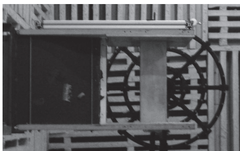
Figure 1: Side view of the experimental set-up showing a NACA 0012 airfoil placed in the open-jet anechoic wind tunnel of ECL.
