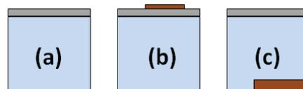
Figure 1. Plate-cavity coupled problems for SmEdA analysis: (a) Bare plate coupled to cavity. (b) Damped plate coupled to cavity. (c) Bare plate coupled to damped cavity
