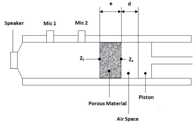
Figure 3. Impedance tube measurement of the "two-cavity-method"
