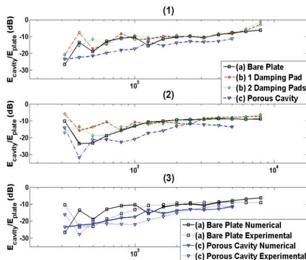
Figure 12. Subsystem energy ratio ( $E_{cavity}/E_{plate}$ ) in 1/3 octave bands for case (a), (b) and (c). (1) SmEdA predictions. (2) Experimental results. (3) Comparisons between SmEdA prediction and experimental results for case (a) and (c).
