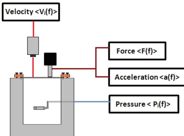
Figure 8. Experimental setup of the plate-cavity coupled structure. Subsystem frequency responses (plate velocity and cavity pressure) are simultaneously measured as the plate is excited. Force and acceleration at the drive point are also measured with an impedance head.
