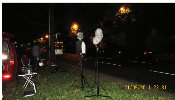
Figure 5: Measuring equipment installed on site (from right to left, Soundfield microphone, Neumann artificial head, radar station and B&K measurement microphone).
