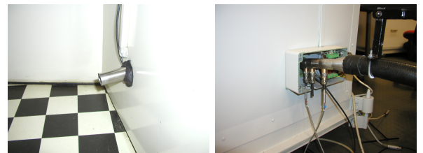
FIGURE 18 – Constant Volume Velocity source mounting : Monopole
