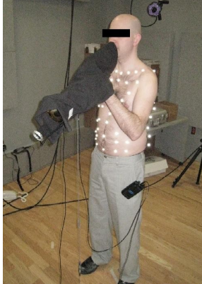
Figure 1: Subject 3 with the 89 reflective markers during measurements. The trumpet is covered by a black bag to avoid reflective perturbations from the instrument.
