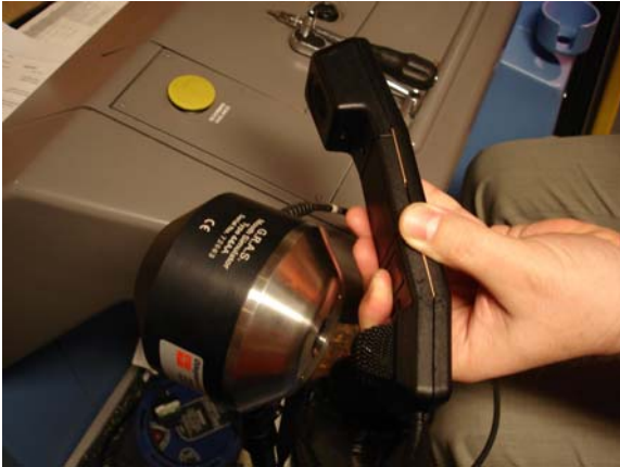
Picture 2: Mouth simulator used with the driver’s handset
