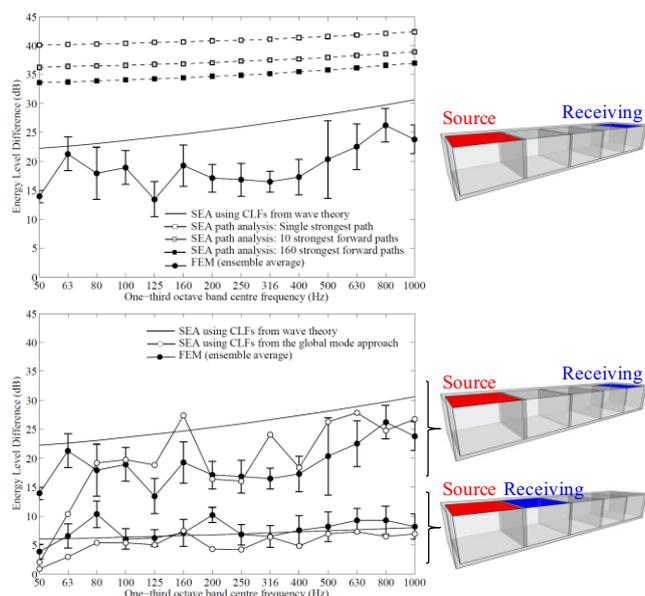
Figure 5: Energy level difference between floors predicted using FEM and SEA. Upper graph shows SEA with coupling loss factors from wave theory for matrix and path analysis. Lower graph includes SEA when calculating coupling loss factors from a global mode approach.
