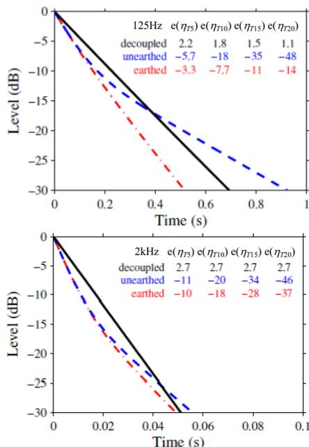
Figure 2: TSEA structural decay curves for the test element along with the percentage errors in the total loss factors.
