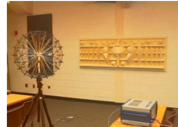
Figure 7: Acoustic Camera set-up and acoustic wall panels
