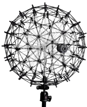
Figure 1: 3D-microphone array with 120 spherically distributed microphones for three-dimensional acoustic analysis.
