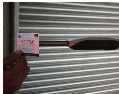
Figure 5: Accurate microphone positioning using lasers.
