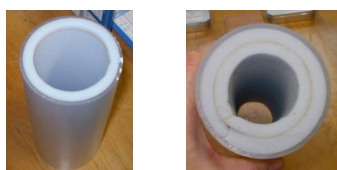
Figure 5: Test duct with melamine foam: (left) \delta = 10 \text{ mm} and (right) \delta = 20 \text{ mm} .
