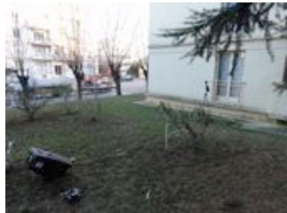
Figure 3. Example of façade sound insulation measurement in accordance with NF EN ISO 10052.
