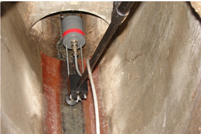
Figure 7: The method for sensor deployment in a live (300mm) sewer in the field.
