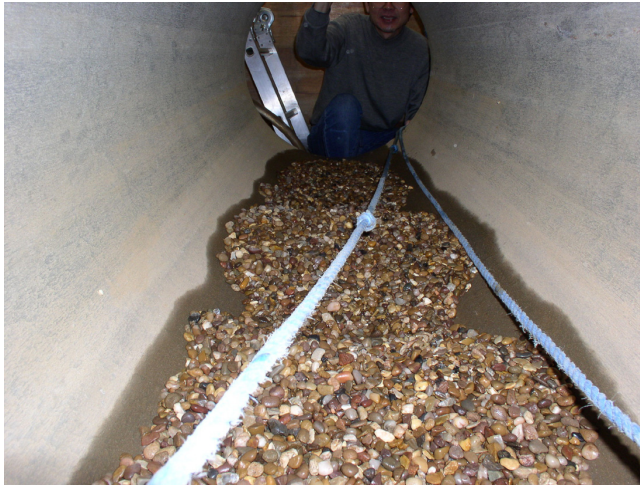
Figure 6: The method for sensor deployment in a live (300mm) sewer in the field.
