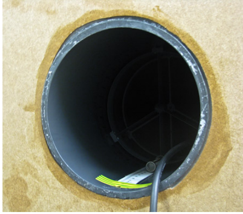
Figure 2: Microflow USP probe, fixed to a frame and inserted into the open end of the pipe
