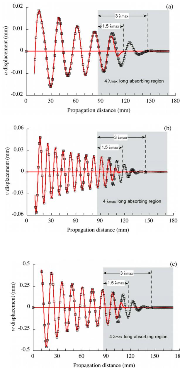
Fig. 6: Comparison between mode attenuations using (—) new AR and (-□) classical AR:  $S_0$  mode (a),  $A_0$  mode (b), and  $SH_0$  mode (c).
