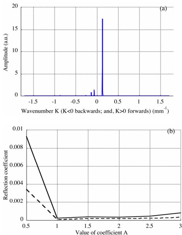
Fig. 4: Optimization of AR with 5mm thick aluminium plate using monitored  $u$  displacement of  $S_1$  mode incident at frequency 0.6MHz, (a) Fourier transform result of  $u$  displacement,  $A=3$ ,  $\beta=0.5$ ; (b) calculated reflection coefficients for optimum coefficient  $A$  with  $\beta=1.5$ , (—) and (---) for the two biggest reflected modes, respectively.
