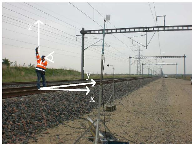
Figure 1: Position of the acoustic source on the experimental site.
