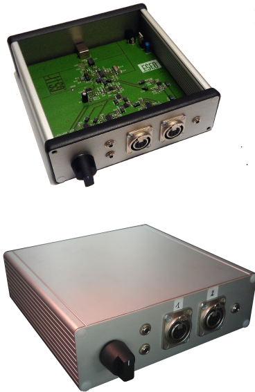
Figure 5: Prototype 2011 of the signal acquisition device of the PAFI project (picture: R. Féron, GSII-ÉSÉO).
