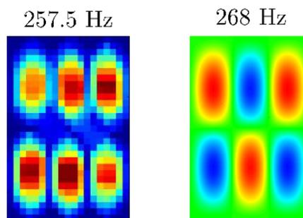
Figure 8: Example of comparison between the sixth soundboard mode found with experiment and with numerical model.
