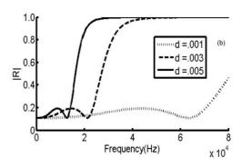
Figure 2: Effect of thickness on frequency dependence of a plane sound wave incident at  $60^{\circ}$  on a 6mm APPM layer of  $BaTiO_3$ .
