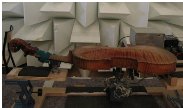
Figure 3 : Positioning of the violin for the back response measurement
