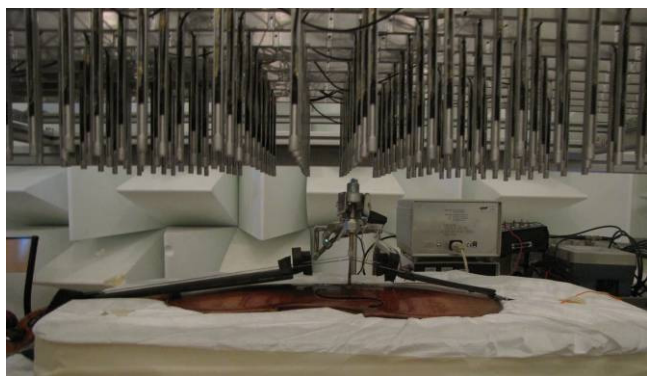
Figure 2 : experimental set up for the soundboard response
