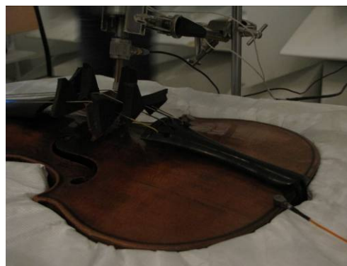
Figure 4 : muffling system, excitation and reference accelerometer
