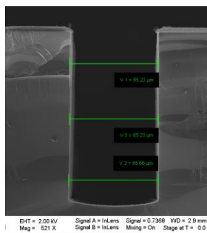
Fig 3. SEM image: cross section of microfluidic channel
