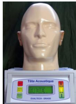
Figure 3: Acoustic head used for measuring acoustic level of music players.
