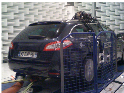
Figure 10: Peugeot 508 on a roller bench.
