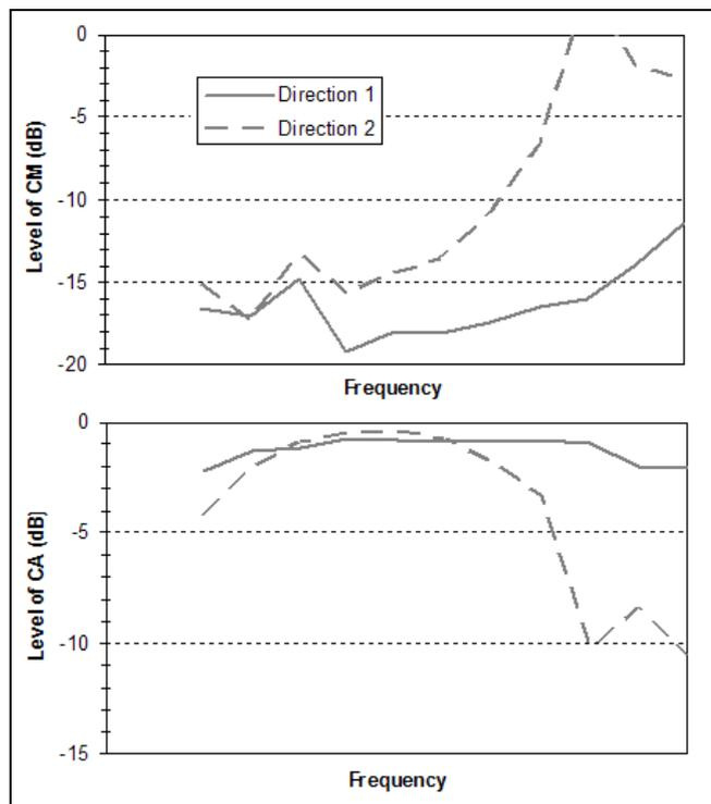
Figure 8: Decoupling and anechoism coefficients of test panel
