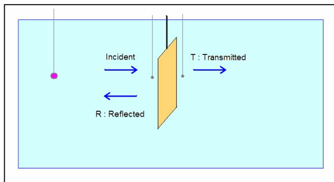
Figure 1: Test panel measurement in a water tank
