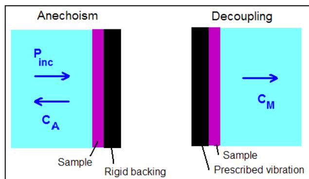
Figure 2: Definition of anechoism and decoupling coefficients
