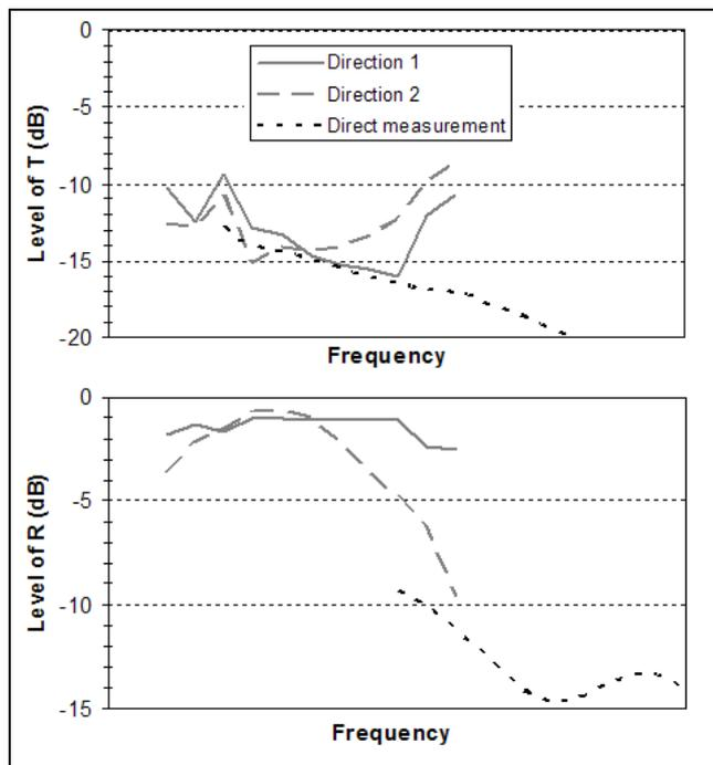
Figure 9: Transmission and reflection coefficients of test panel on a steel backing plate
