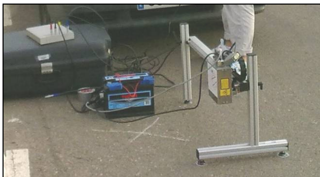
Figure 4. LaserStaticPG-LA 2 IC used for the profile measurements of the pavement surfaces.
