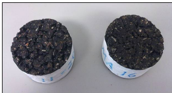
Figure 5. Samples studied. SMA 11 3c CF (Left) and SMA 16 3c CF (Right).
